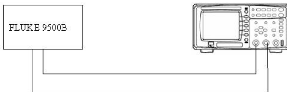
Picture 3-1 Connecting test instruments
